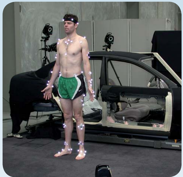
One of the subjects fully kitted out in all the sensors needed to collect data for the AutoCRC Ingress/Egress Project.
