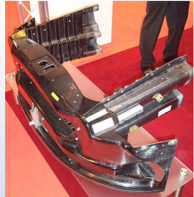
Aston Martin Vanquish composite crash structure*
